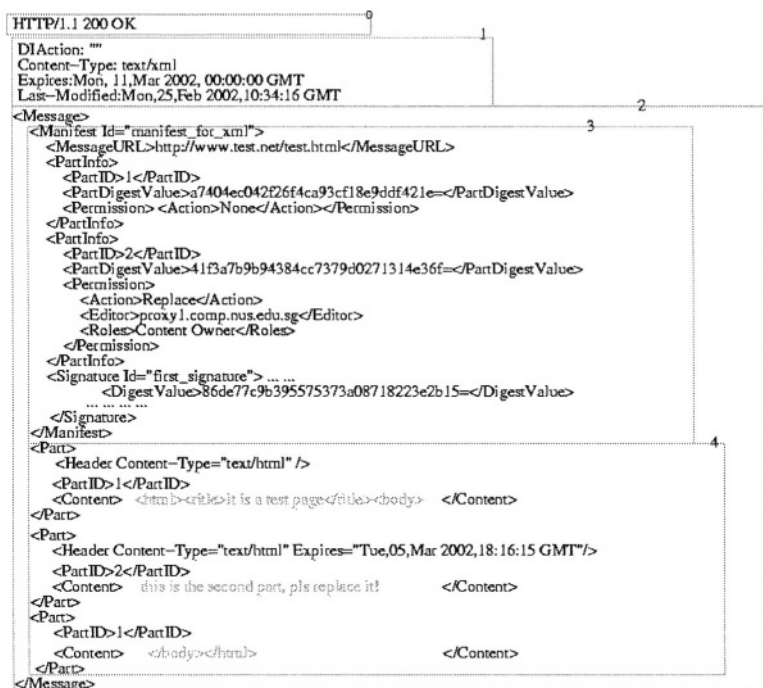
Fig. 2. Data-Integrity Message in a Server
