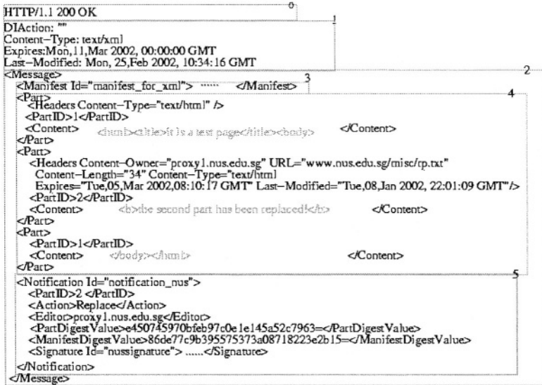
Fig. 3. Data-Integrity Message after the Modification by a Web Intermediary
